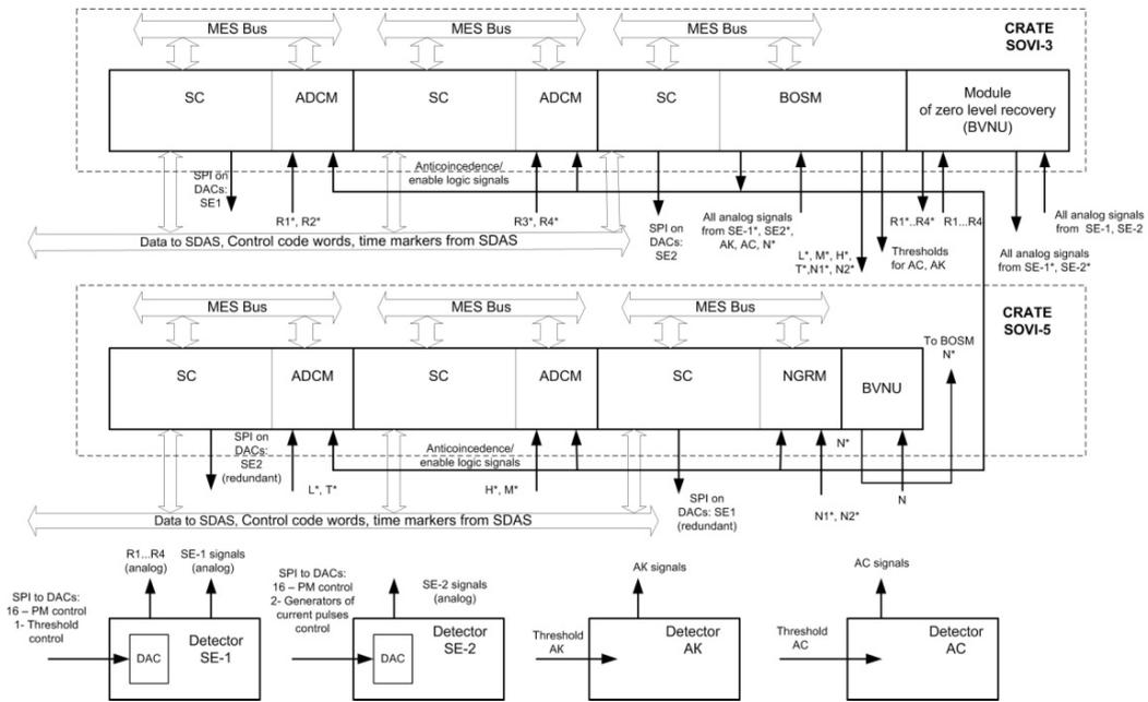
Fig.3. Block diagram of NATALYA-2M electronics (output signals from BVNU are marked by symbol \*).
