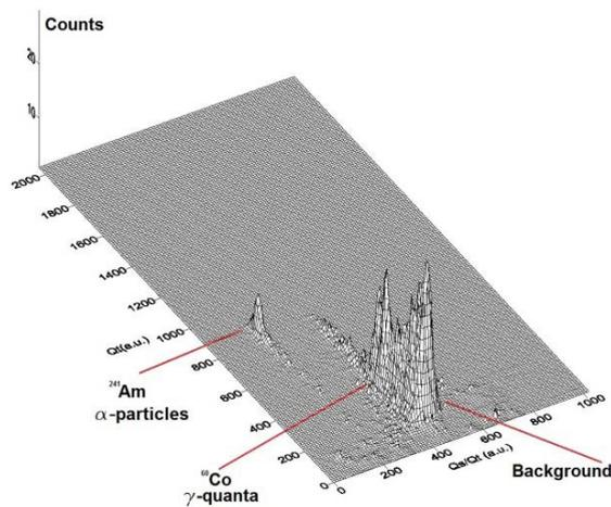
Fig. 6. Example of  $^{241}\text{Am}+^{60}\text{Co}$  3D  $Q_{slow}/Q_{tot}$  versus  $Q_{tot}$  distribution, measured by ADCM module in Regime 3.
