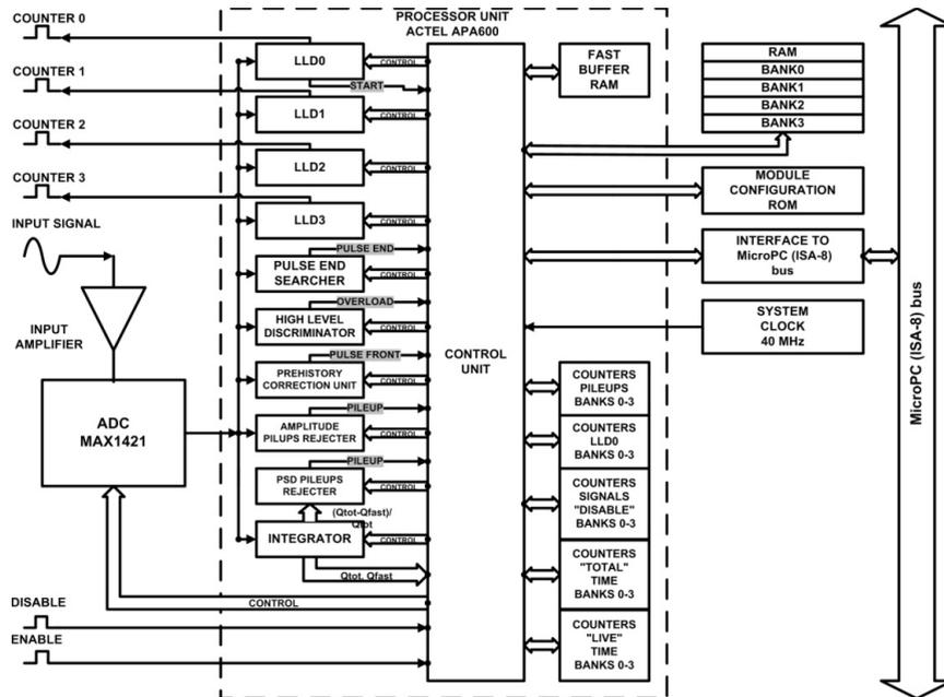
Fig.4. Functional diagram of ADCM module channel (only main counters are shown). Output signals COUNTER 0-3 arrive to external counters.
