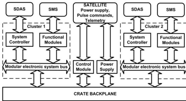
Fig. 1. Functional diagram of two-cluster configuration.
