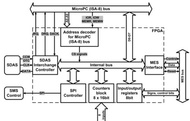
Fig. 2. Functional diagram of system controller module.
