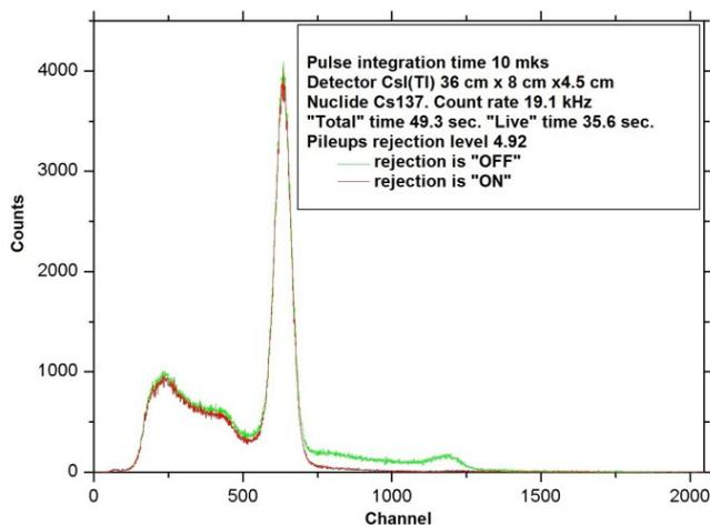
Fig.5. Example of  $^{137}\text{Cs}$  spectrum, measured by ADCM module in Regime 2 with and without amplitude pileups rejection.
