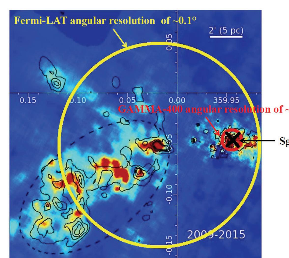
Comparison of the capabilities to study Galactic Center by Fermi-LAT with the angular resolution of ~0.1° for  $E_{\gamma} = 100$  GeV (yellow circle) and **GAMMA-400** with the angular resolution of ~0.01° for  $E_{\gamma} = 100$  GeV (red circle), using Chandra X-ray observation. The Sgr A\* position is marked by cross.
