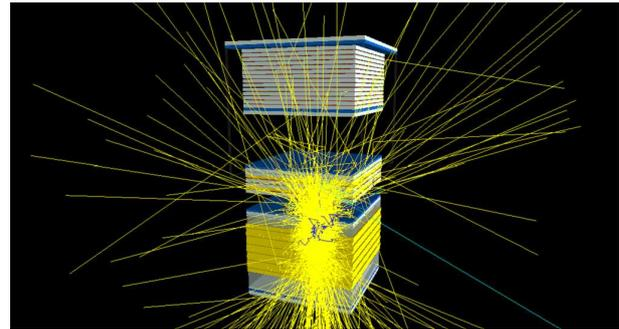
**Figure 2.** The interaction of the 100-GeV gamma ray with the GAMMA-400 matter with the formation of backscattering particles. Secondary gammas, positrons and electrons are marked by yellow, violet and blue colors respectively
