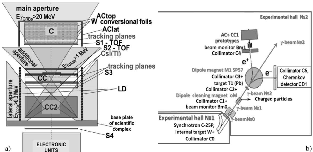
**Figure 1.** The physical schemes: a) of the under consideration variant of GAMMA-400 gamma-ray telescope construction and its three apertures for GRBs registration, b) positron beam formation setup and apparatus installation at C-25P synchrotron “PAKHRA”.
