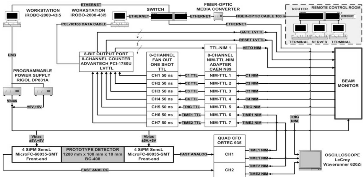
**Figure 3.** Functional diagram of the data acquisition.
