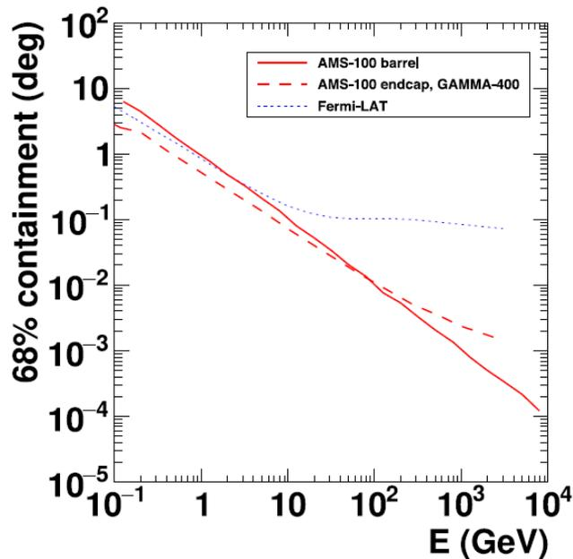
GAMMA-400 calculated angular and energy resolutions vs energy.
