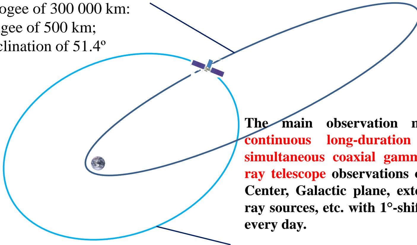
Under the action of gravitational disturbances of the Sun, Moon, and the Earth after ~6 months the orbit will transform to about circular with a radius of ~200 000 km and will be without the Earth's occultation and out of radiation belts.
