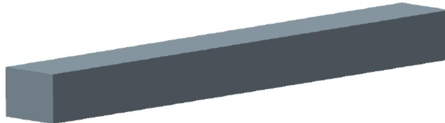
Crystal dimensions are  $400 \times 50 \times 37 \text{ mm}^3$
