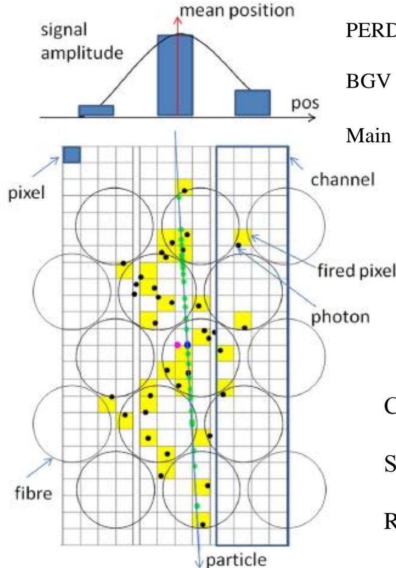
Channel width is 250 μm
