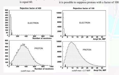
To take into account the fact that the hadron cascade begins to develop deeper inside the instrument, than the electromagnetic shower, the signals in detector systems CC1, S2 and S3 are considered. For protoninduced cascades, there are a lot of events with small signal amplitude.
