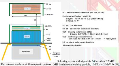
AC - anticoincidence detectors (AC top , AC lat) C - Converter-Tracker - total 1 Xo 8 layers W 0.1 Xo +Si (x,y) (pitch 0.1mm) 2 Si(x,y) no W S1, S2 - TOF detectors
