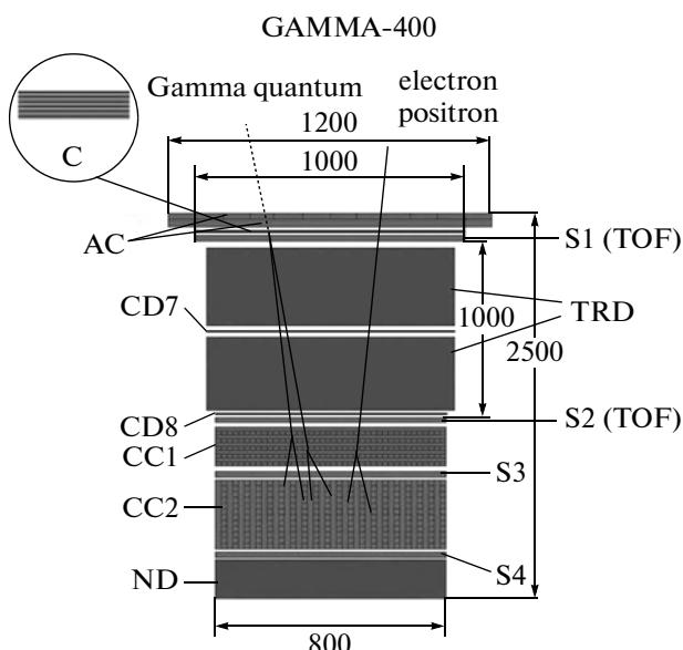
**Fig. 1.** Physical scheme of the GAMMA-400 gamma-ray telescope.
