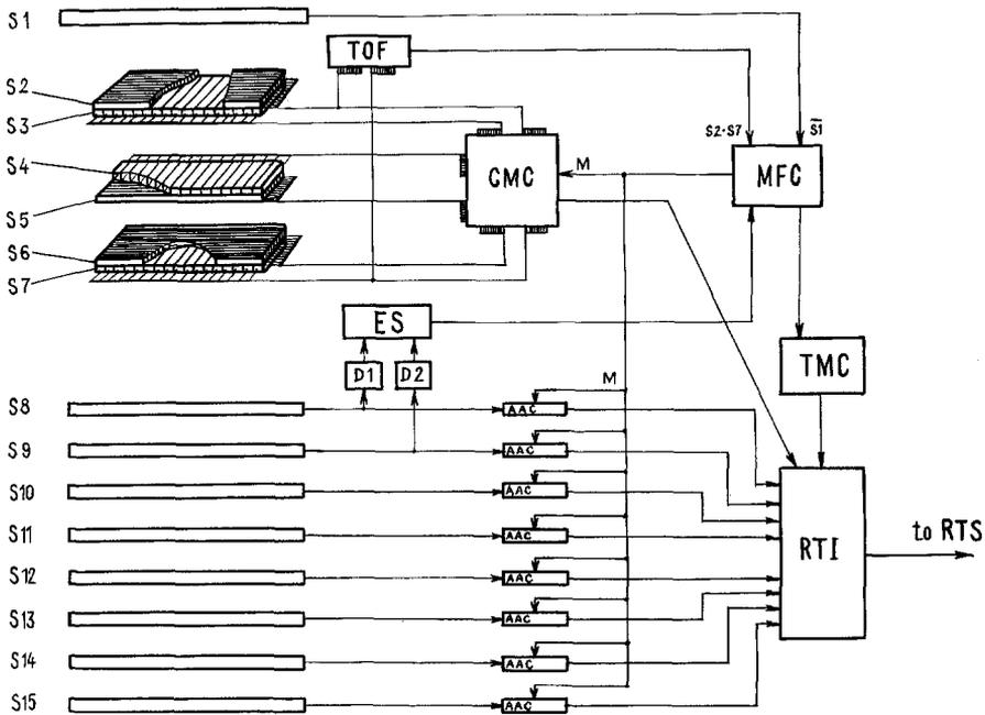
Fig. 6. Block diagram of the GAMMA-400 electronics. S1-S15: scintillators of the detecting block; D1 and D2: discriminators; ES: energy measurement circuit; TOF: time-of-flight circuit; MFC: master formation circuit; M: master signal; CMC: coordinate measurement circuit; TMC: time measurement circuit; AAC: amplitude analyzer circuit; RTI: radio-telemetry interface; RTS: telemetry system.
