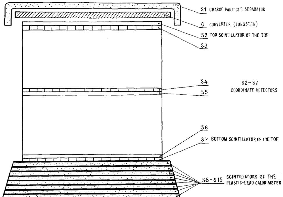
Fig. 5. Scheme of the detecting block of GAMMA-400.
