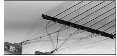
Fig. 6. Scintillator light gathering in the PS layer using WLS fibers.
