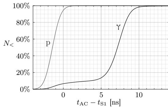
Figure 5: Cumulative distribution functions of S1-to-AC lag. Value of  $N_{<}$  at abscissa  $t$  refers to fraction of events where the lag is less than  $t$ . Both gamma rays and protons are plotted.
