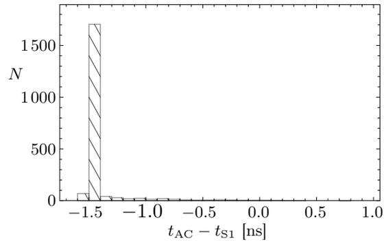
Figure 3: Distribution of the difference between AC and S1 when detecting protons (note expanded horizontal scale)
