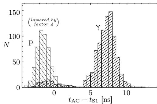
Figure 4: Normally blurred distribution of the difference between AC and S1 triggerings when detecting gamma rays and protons. Standard deviation of the blur is a pythagorean sum of AC and S1 time resolutions. For convenience of comparison, heights of columns on proton histogram are lowered fourfold.
