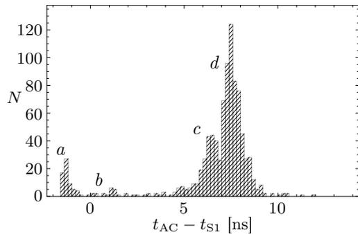
Figure 2: Distribution of the difference between AC and S1 triggerings when detecting gamma rays; *a*: conversion in AC, *b*: backplash from C, *c*: from CC1, *d*: from CC2,
