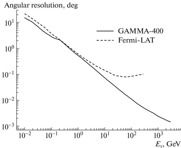
**Fig. 2.** Energy dependence of the angular resolution of the GAMMA-400  $\gamma$ -ray telescope. The analogous dependence for Fermi-LAT is shown for the sake of comparison.
