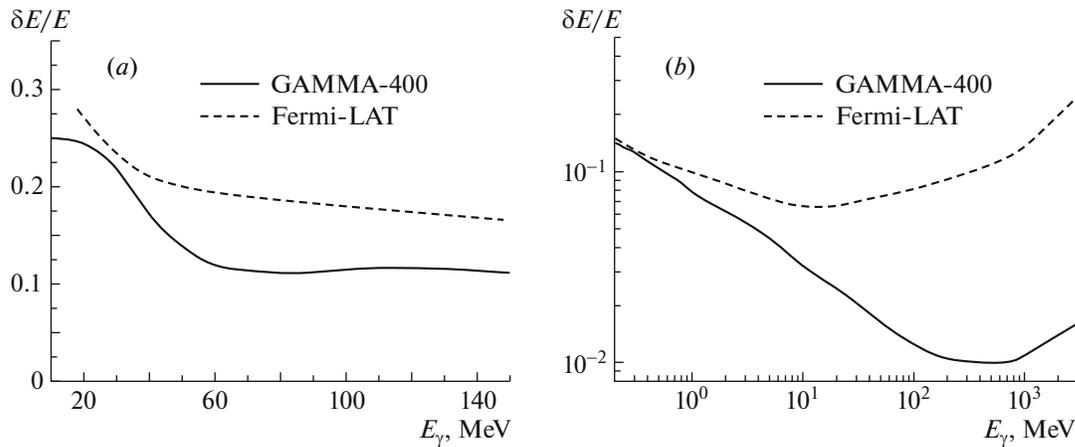
**Fig. 3.** The energy resolution of the GAMMA-400  $\gamma$ -ray telescope as a function of the gamma-ray energy in the ranges of (a) 20–140 MeV and (b) 0.2–1000 GeV. The analogous dependences for Fermi-LAT are shown for the sake of comparison.
