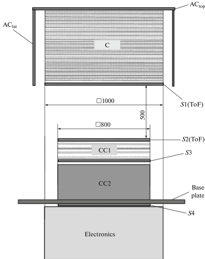
**Fig. 1.** Layout of the GAMMA-400  $\gamma$ -ray telescope: anticoincidence system (AC) (top and lateral detectors), converter-tracker (C), time-of-flight system (ToF), parts of coordinate-sensitive calorimeter (CC1 and CC2), and scintillation detectors of the calorimeter (S3 and S4).
