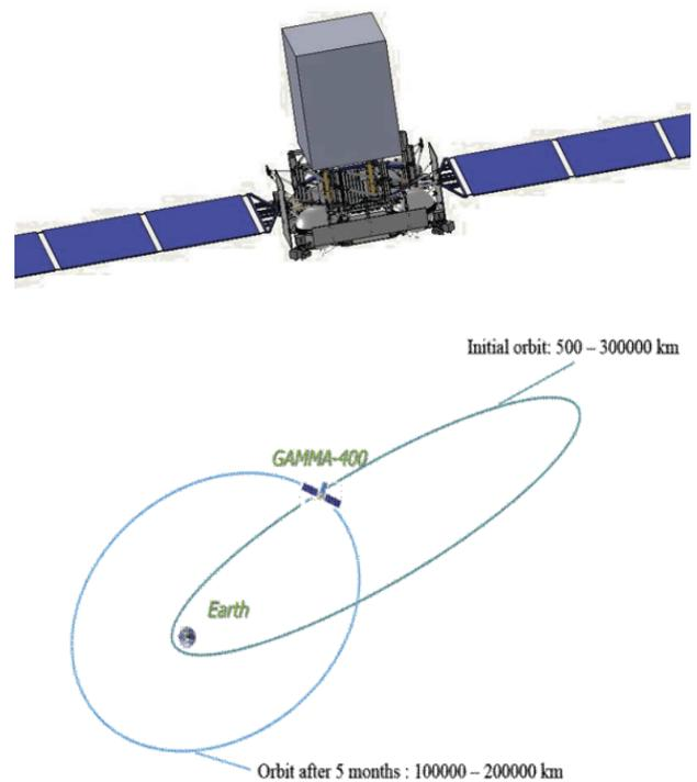
Figure 1: Top: the “Navigator” spacecraft; the gray box represent the GAMMA-400 apparatus. Bottom: the GAMMA-400 planned orbits.
