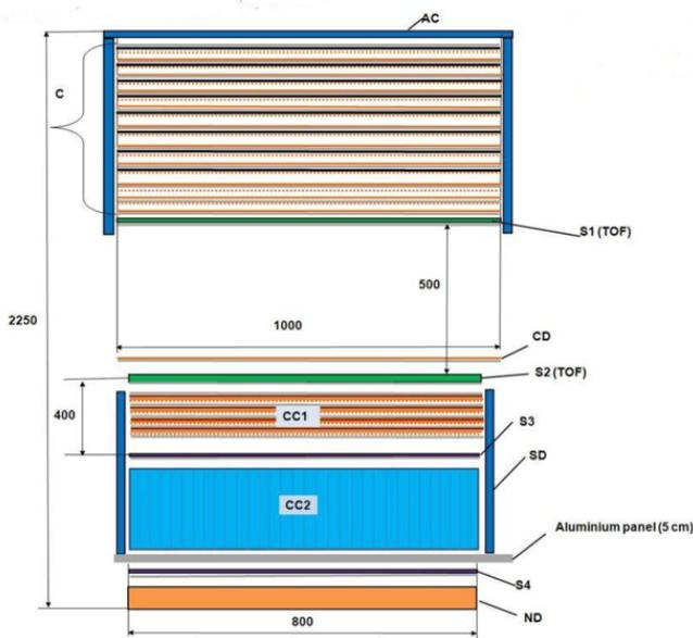
Figure 2: The GAMMA-400 instrument, schematic view of the “baseline” proposal. Where not otherwise stated, lengths are expressed in mm.
