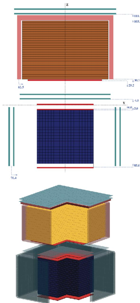
Figure 4: Top: schematic view of a preliminary GAMMA-400 upgraded version. Bottom: 3D view of the same geometrical version, to be noticed the cubic calorimeter made of CsI small cubes.
