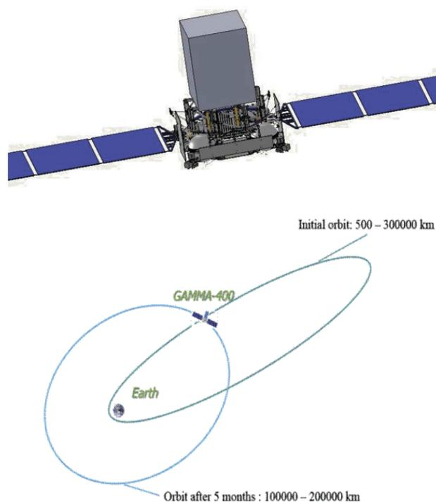
Figure 1: Top: the “Navigator” spacecraft; the gray box represent the GAMMA-400 apparatus. Bottom: the GAMMA-400 planned orbits.
