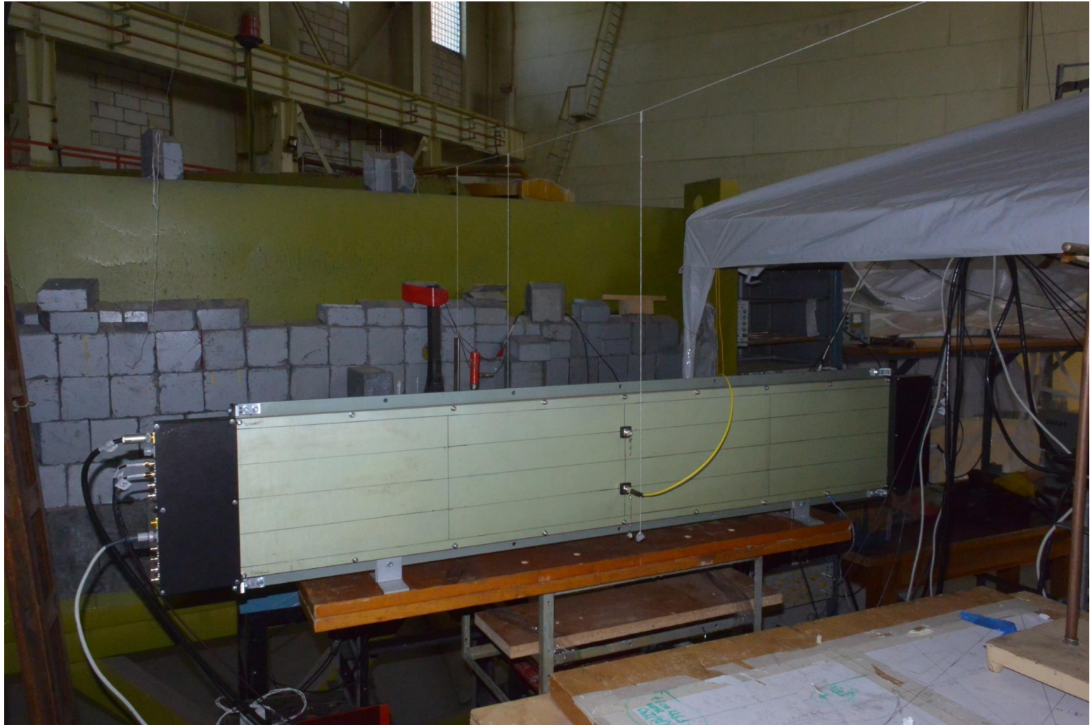
Prototype of AC detector. L = 1300 mm, time resolution is \sim 200 ps, efficiency is 0.999 (A.I. Arkhangelskiy+ ,2020. 2022 in press)
