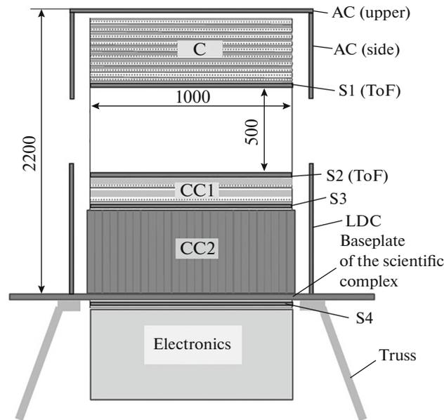
**Fig. 1.** Physical layout of the GAMMA-400  $\gamma$ -ray telescope:  $AC_{top}$ , upper anticoincidence detector;  $AC_{lat}$ , lateral anticoincidence detector; C, converter/tracker; S1 (ToF) and S2 (ToF), scintillation detectors of the time-of-flight system; CC1 and CC2, coordinate-sensitive calorimeter; S3 and S4, scintillation detectors; LDC, lateral detectors of the calorimeter.
