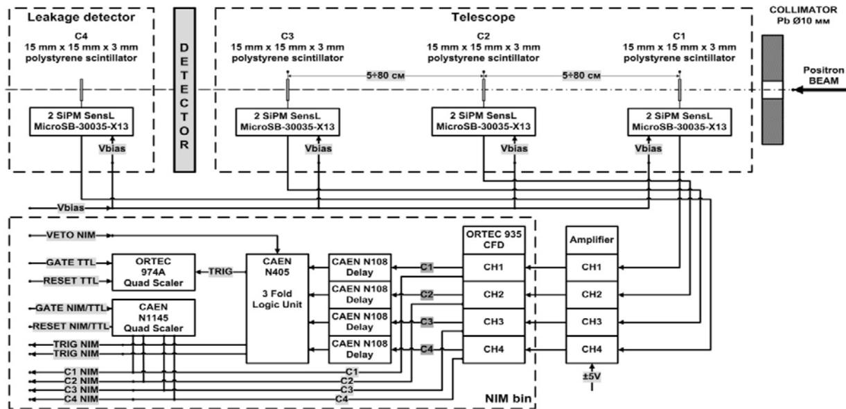
**Figure 2.** Experimental setup, including beam monitor. The dash-dotted line represents the beam line.
