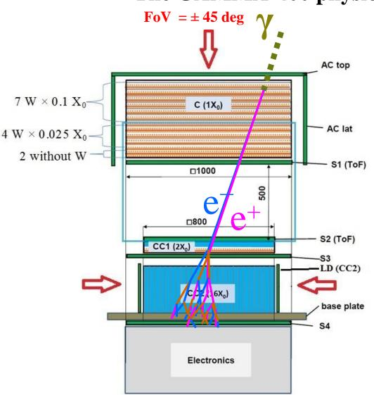
AC – anticoincedence system C - converter-tracker  $\sim 1 X_0$ S1, S2 – TOF detectors CC1, CC2 – calorimeter vertical thickness  $\sim 2+16=18 X_0$ CC2 – lateral thickness  $\sim 43 X_0$ S3, S4 – scintillation detectors
