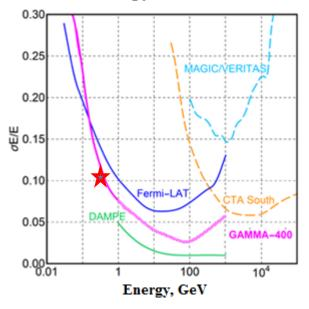
GAMMA-400 calculated angular and energy resolutions vs energy. ★ GAMMA-400 experimental energy resolution for the energy of 300 MeV
