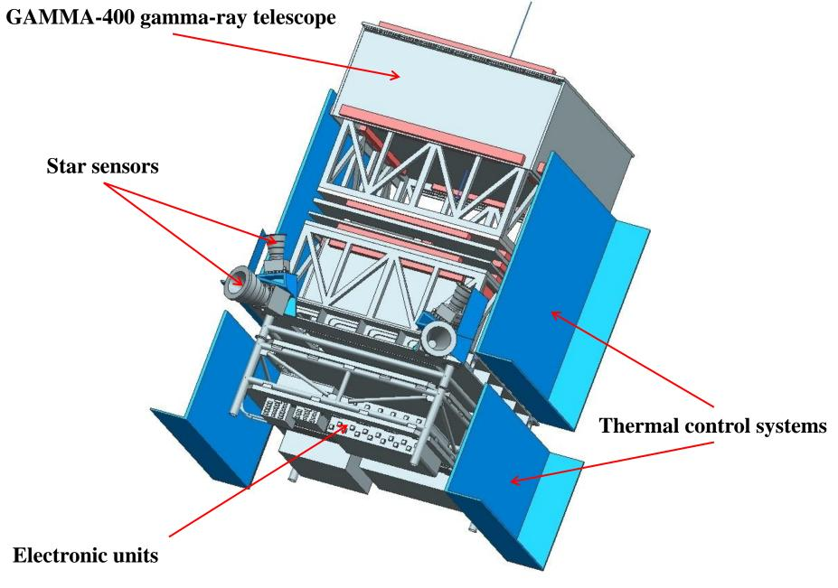
GAMMA-400 gamma-ray telescope
