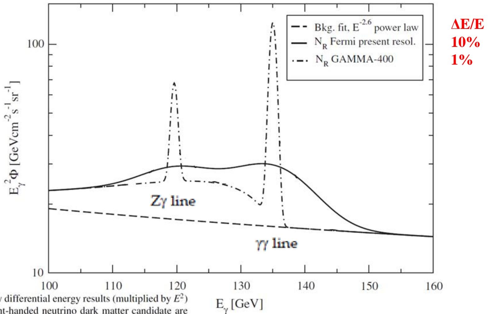
FIG. 3. The  $\gamma$ -ray differential energy results (multiplied by  $E^2$ ) for a 135 GeV right-handed neutrino dark matter candidate are shown, with the present Fermi-LAT energy resolution  $\Delta E/E = 10\%$  FWHM (solid line)
