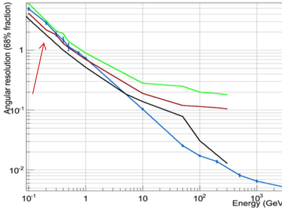
*Point Spread Function results obtained at normal incidence with a more conservative cut on the reconstructed events. Fermi-LAT total Pass7\_V6 (Green), Fermi-LAT front Pass7\_V6 (Red), GAMMA-400 E2 (Black) and GAMMA-400 B2 (Blue).*
