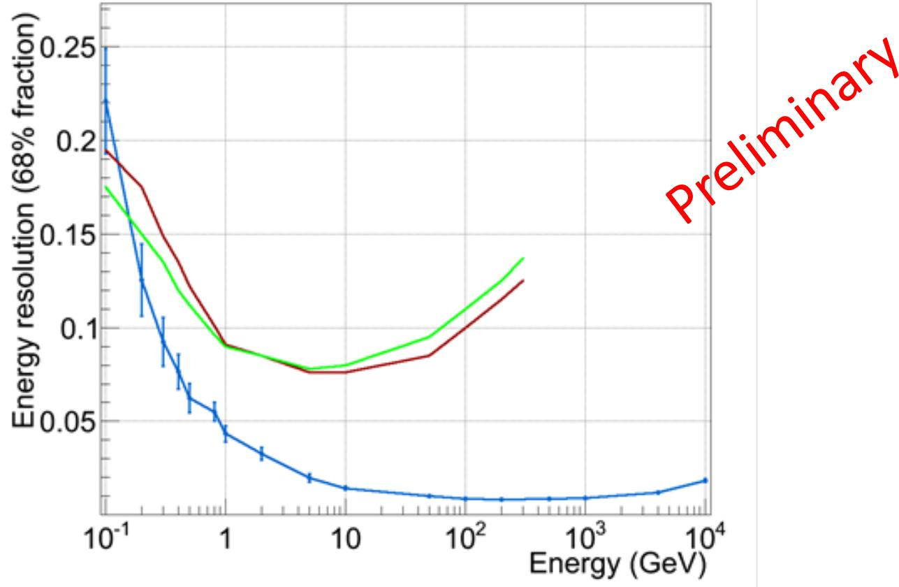
Variation of energy resolution (68% fraction) of the G-400 instrument with B2 configuration with energy for normal incidence and flat area distribution, and comparison with Fermi-LAT. (Blue: G-400, Green: Fermi-LAT total, Red: Fermi-LAT front)
