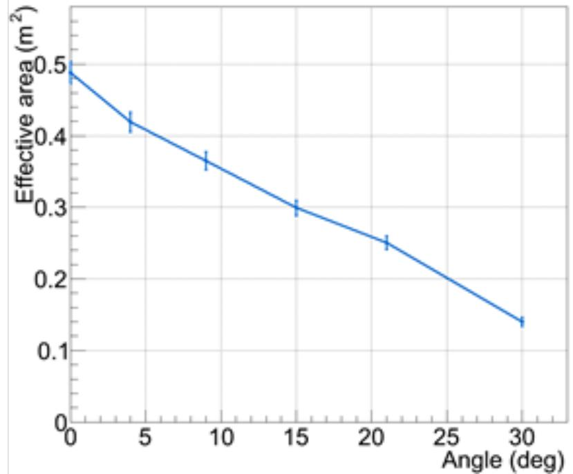
*Effective area ( $m^2$ ) of the G-400 instrument with B2 configuration. Left panel: variation of the effective area with energy for normal incidence and flat area distribution (Blue: G-400, Green: Fermi-LAT total, Red: Fermi-LAT front). Right panel: variation of effective area of G-400 at 100 GeV with polar angle for flat area distribution.*
