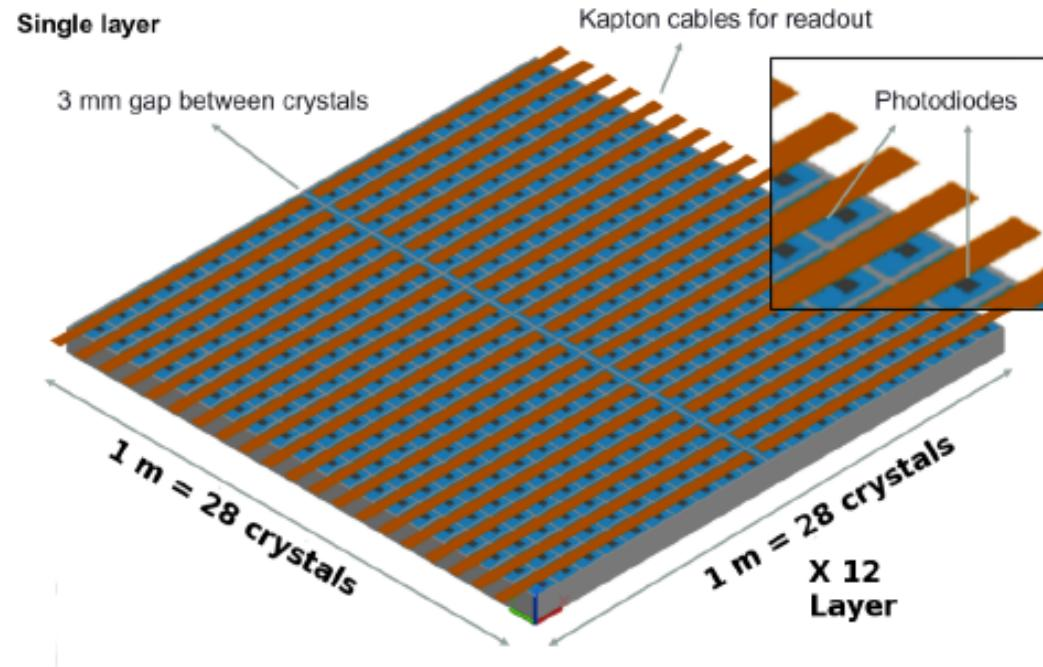
At least 2 photo diodes per crystals to cover the huge dynamical range ( $1\text{-}10^7$  MIP)
